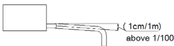
Figure 3-5.1: Drain piping minimum slope requirement
